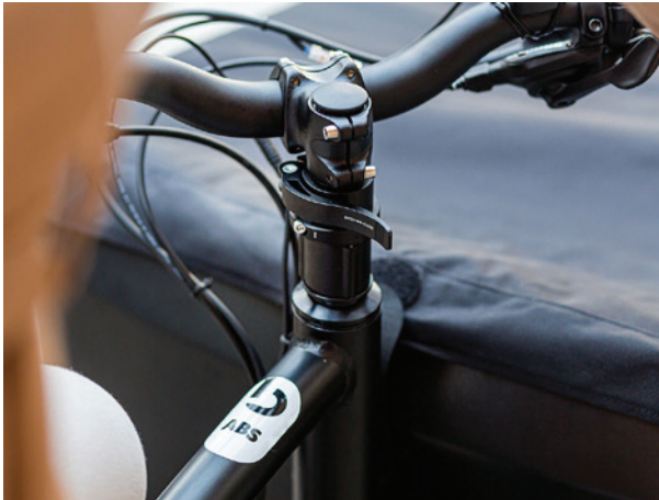
Blubrake's Integrated ABS System for e-Bikes.
