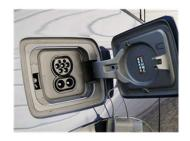
Typical Combined Charging System (Combo 2) vehicle inlet
